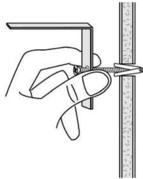
Pull back on assembly to hold the wings inside the wall to prevent the wings from spinning while tightening bolt. Turn the bolt with the screwdriver until firmly tightened.
