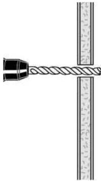
Insert the bolt through the fixture to be fastened, thread on wings, then fold the wings completely back and insert through the hole until wings spring open.
