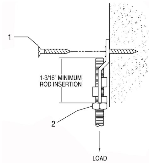
1. Screw hanger directly into structure.
