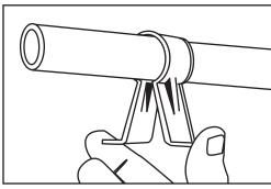
2. Squeeze strap back around pipe Allow pipe to slide back and forth
