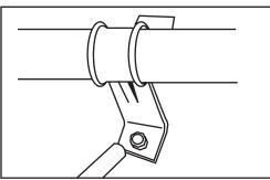
3. Fasten the strap to the wood surface using the two hex head screws provided.
